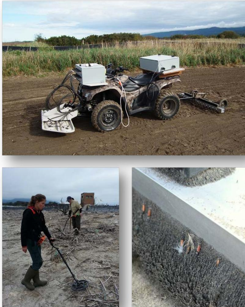
Figure 5. PIT tag detection equipment used on the East Sand Island Caspian tern colony in 2016 included a hand-held portable system (bottom left), an eight-coil flat-plate system attached to an ATV (top), and a towable sweeper magnet attached to an ATV (top and bottom right).
